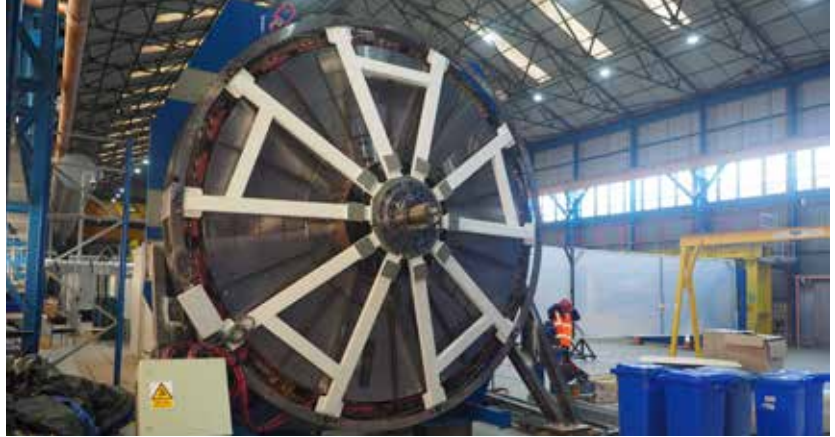
GreenSpur Wind's primary innovation lies in its permanent magnet agnostic generators (PMGs). (Courtesy: GreenSpur)
