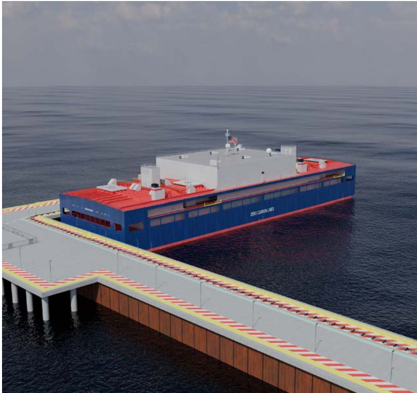
Rendering of a nuclear-powered floating data center from Herbert Engineering (HEC). (Courtesy: ABS)
