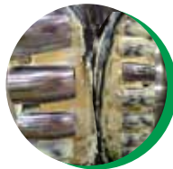
Castrol® Tribol® grease after 3 years of service
