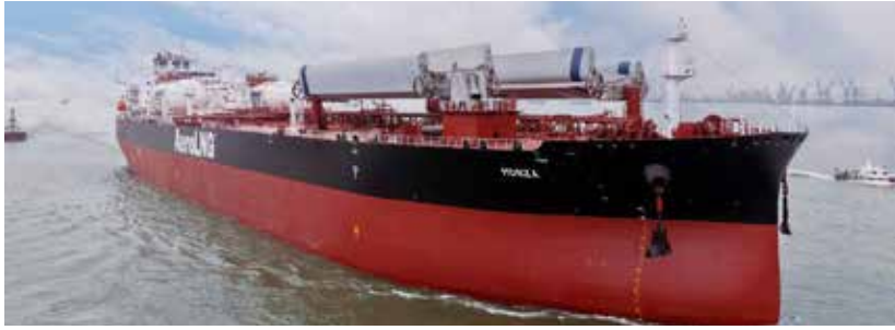
The Monza is an LR2 tanker fitted with two 37.5m WindWings. (Courtesy: Windwings)
