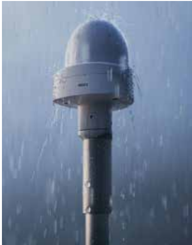
RM60 uses patented radar technology to measure each falling raindrop, snowflake, and hailstone. (Courtesy: Vaisala)
