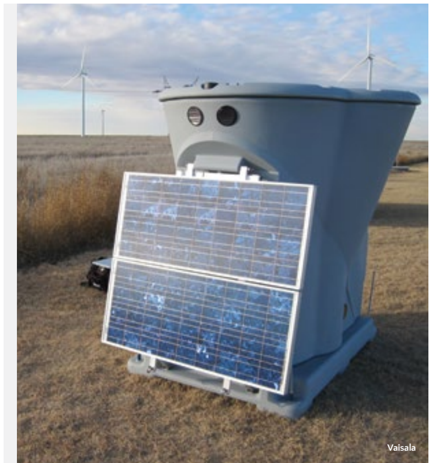
Vaisala's Triton® wind profiler is an advanced remote sensing system that provides accurate wind measurement data across the entire blade sweep of today's largest wind turbines.
