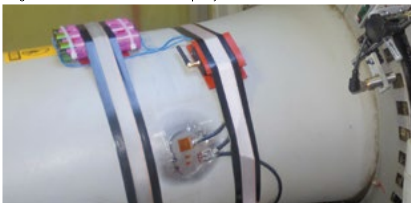
Figure 2: Wind turbine main shaft instrumented with strain gauges
