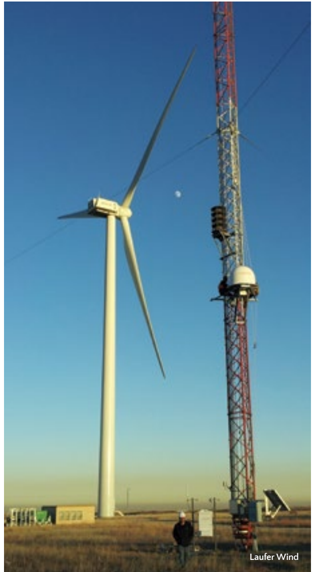
Laufer Wind's dome-covered radar on a Met tower at the National Renewable Energy Laboratory (NREL)
