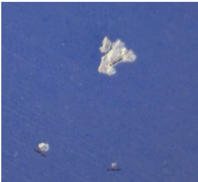
Figure 7: Measurement of defect size on a silicon surface replica
