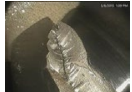
Figure 5: Example of a fractured tooth crack close to full liberation of the damaged area
