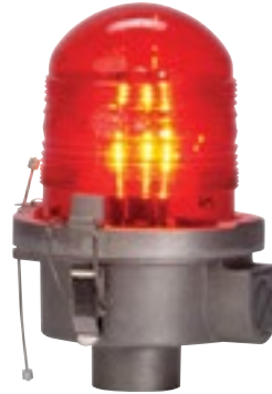
The MKR-LTE1-01R single obstruction light integrates visible red LEDs and infrared LEDs into a single L-810(L). Infrared energy (IR) can enhance compatibility with aviator's night vision imaging systems (ANVIS) and night vision goggles (NVG). Precision-molded Fresnel optics produce a low ground scatter tower lighting solution. The die cast aluminum base provides 3/4-inch conduit hubs for side or bottom mounting. Multiple 9kA MOVs and a 20kA gas plasma discharge tube provide robust surge suppression.
