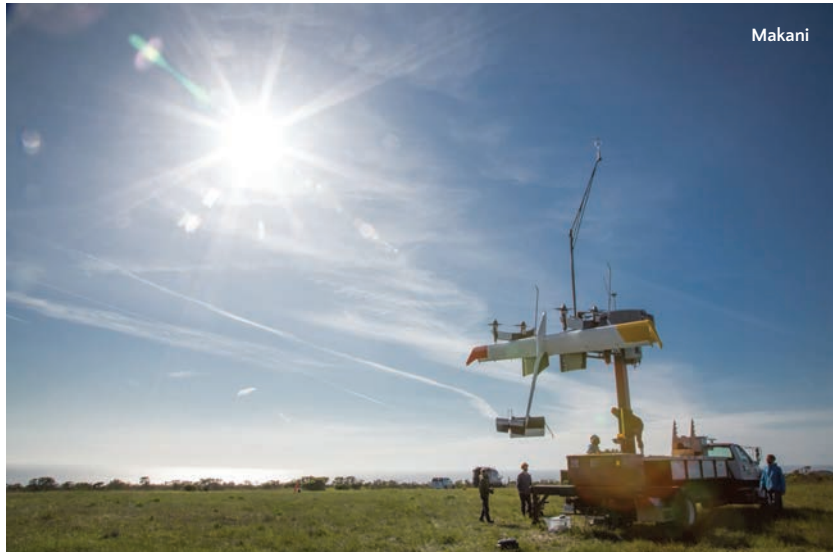
Makani's 30-kW energy kite prototype perched on a ground station prototype at one of the company's test sites in California.
