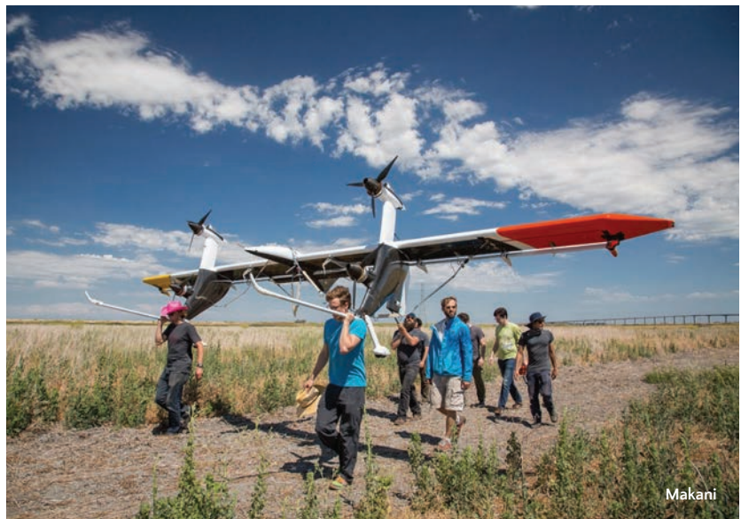
The Makani team hand-carries the 30-kW energy kite prototype back from the ground station after a successful day of field testing.
