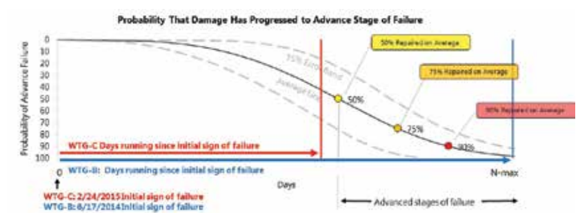
Figure 9: RomaxRepair estimates the remaining useful life once main bearing damage has been detected and confirmed.
