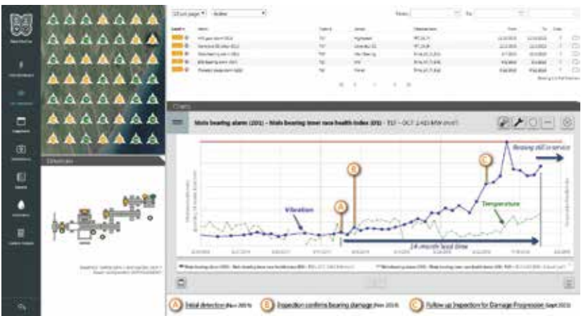
Figure 4: Romax InSight Fleet Monitor™ software tracking main bearing damage provides over a year's leadtime on the failure using advanced algorithms applied to the raw vibration data feed.
