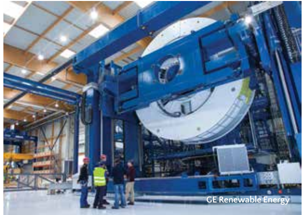
Each generator weighs 150 tons and measures 7.6 meters in diameter.
