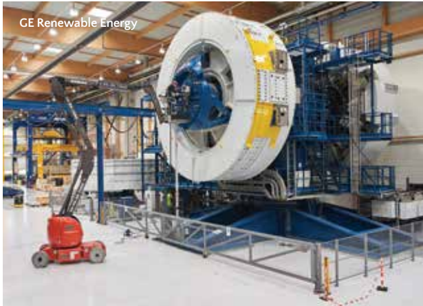
GE builds the permanent magnet generators in the Saint-Nazaire plant.
