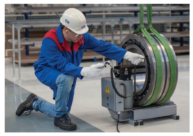
of damage to a bearing, shaft, or workpiece and help increase bearing service life and machine reliability. Ultimately, proper heater selection is critical for application success.
