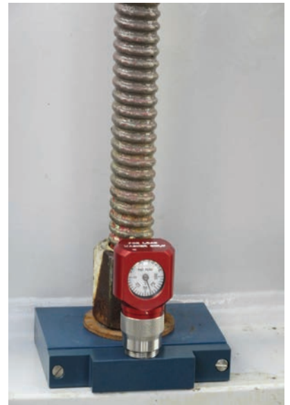
Load-indicating washer with gauge attached confirming the load remained after the tensioning procedure. (Courtesy: Torkworx)
