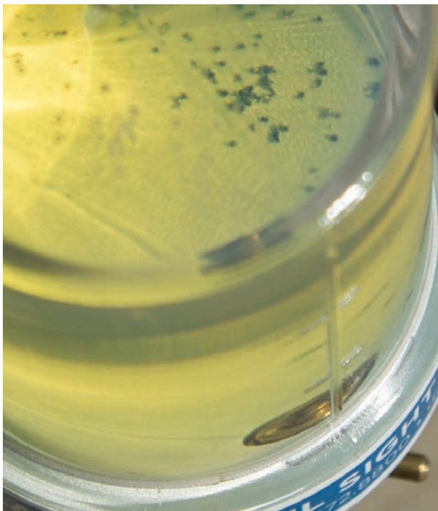
Contamination particulates can be more easily seen against the OSG’s white background. (Courtesy: Des-Case Corporation)
