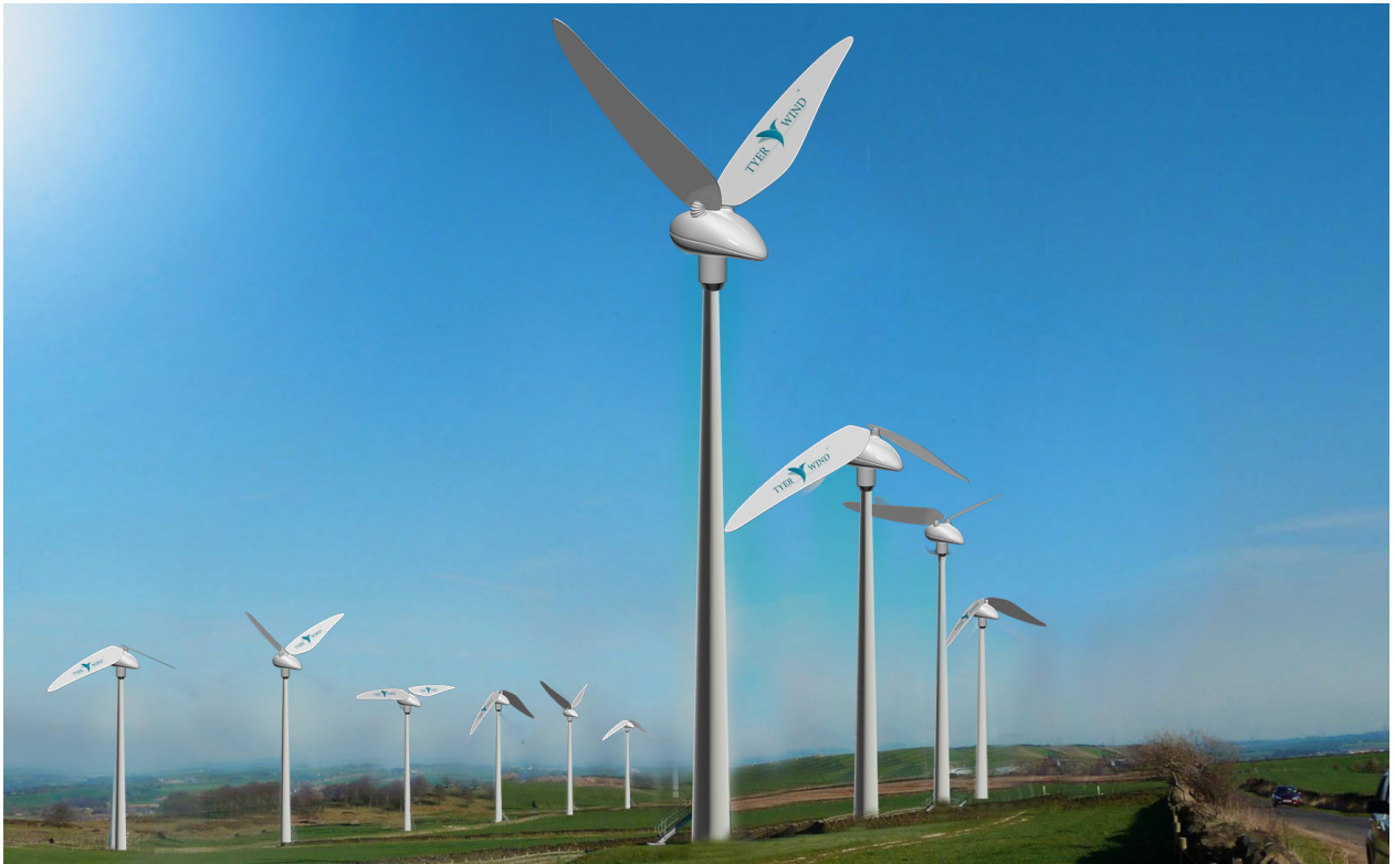
Instead of traditional blades, Tyer Wind's technology would use "flapping wings" that convert wind energy into electricity based on 3D Aouinian Kinematics. (Courtesy: Tyer Wind)
