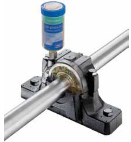
Single-point automatic lubricators inject the precise and correct amounts of contaminant-free grease and often will be used for the re-lubrication of pitch bearings and other bearings in moving parts. (Courtesy: SKF USA)
