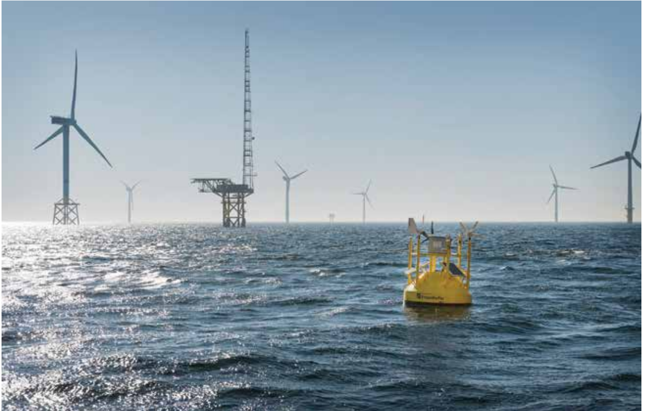
The Fraunhofer IWES LiDAR buoy has already been used multiple times for offshore measuring. (Courtesy: Fraunhofer IWES)
