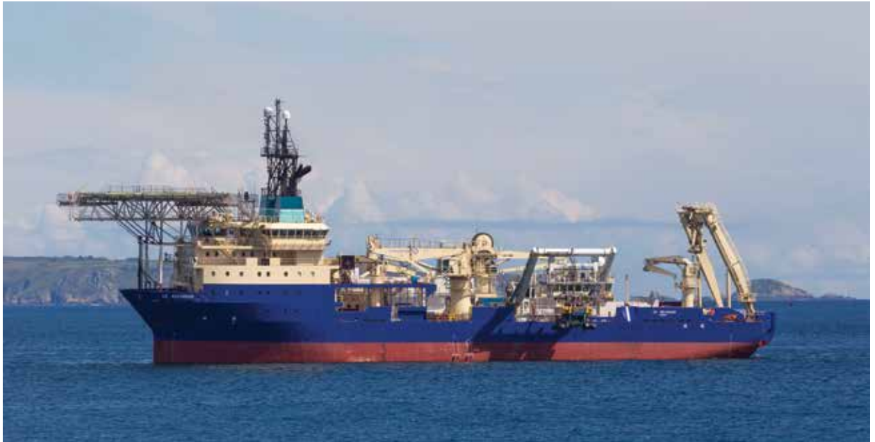
The project used the CS Recorder, which has DP2 dynamic positioning; the Q1000, a powerful remotely operated vehicle (ROV) jet trenching system; as well as a skilled onshore and offshore engineering team. (Courtesy: Global Marine Group)
