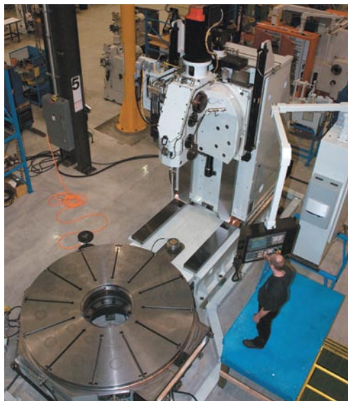
An aerial view of the massive worktable and column being assembled on the plant floor.
