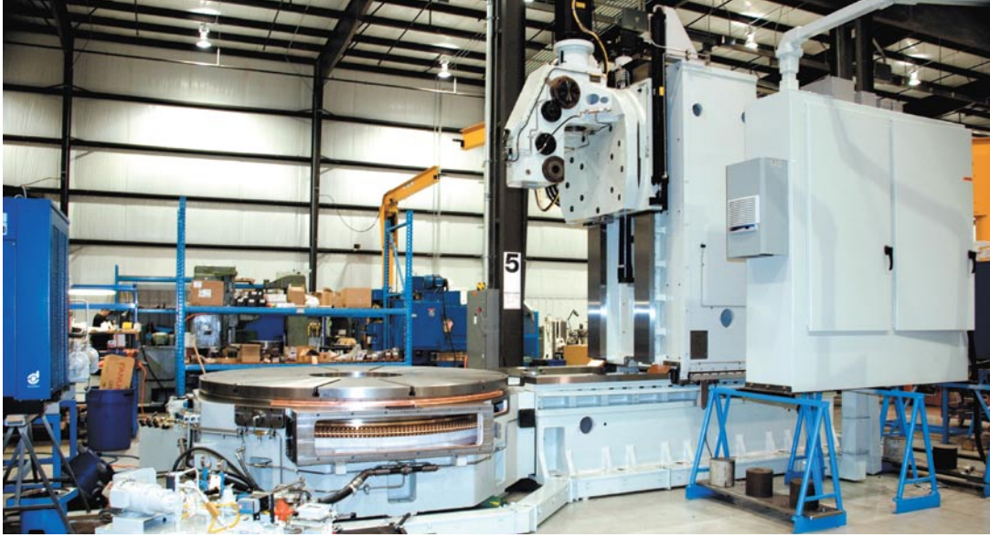
G&E machines can be configured with a single or two columns, with interchangeable cutting heads.
