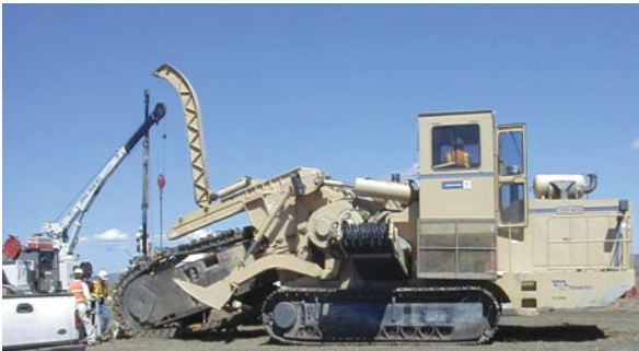
Fig. 6: Maintaining the chain trenching machine.
