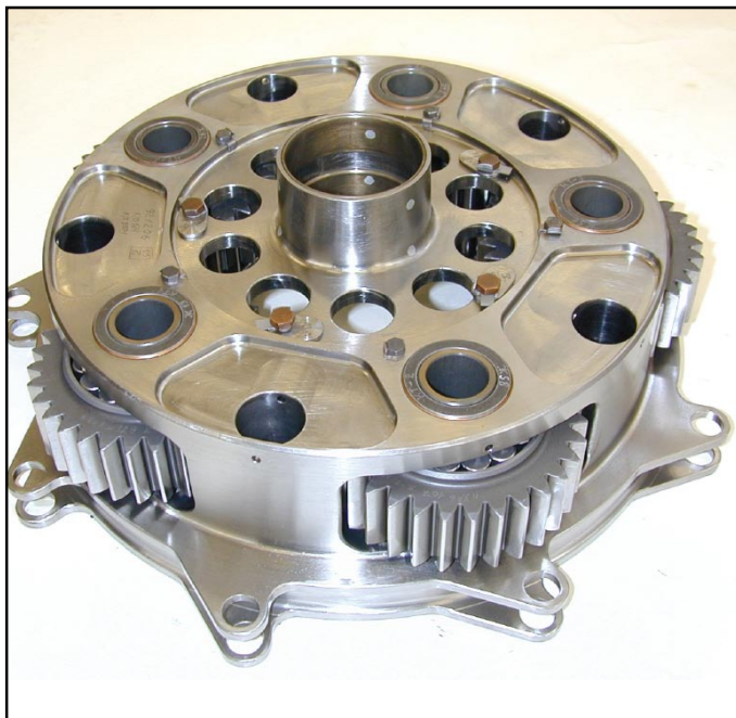
Fig. 3: Example of the asymmetric gear application.
