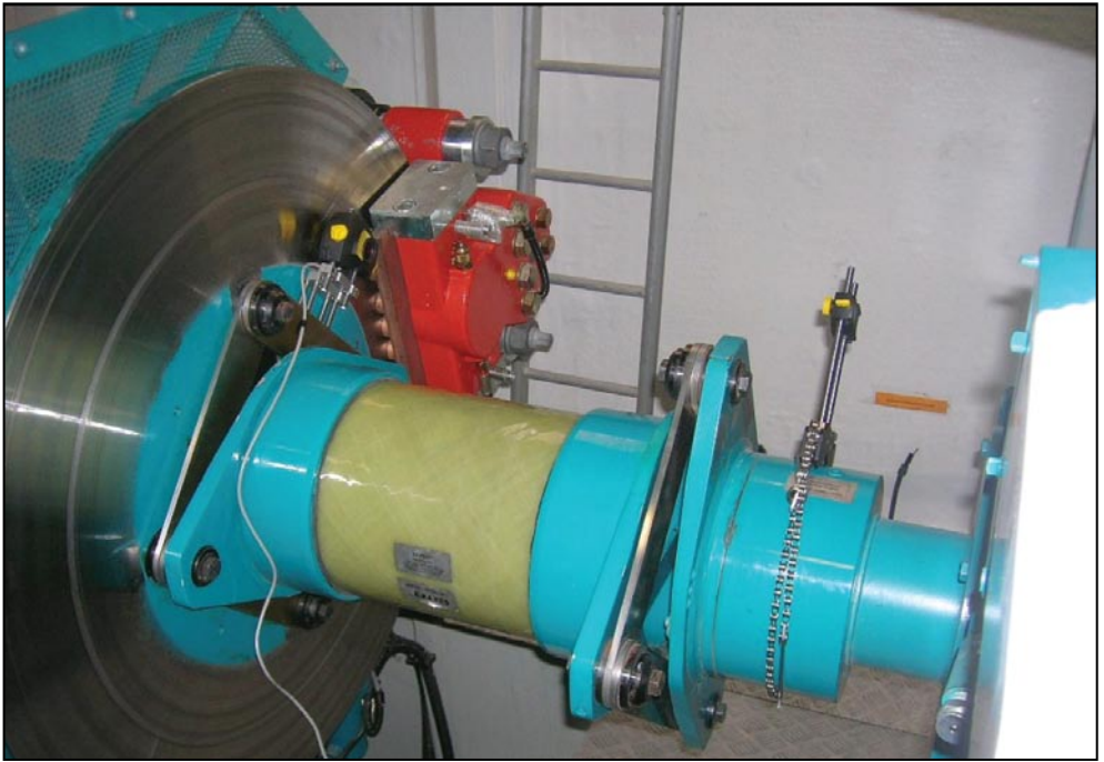
Fig. 5: A laser emitter is mounted on a magnetic bracket with offset adapters directly to the brake disc on a Suzlon gearbox output shaft (Jack Jackson, Alignment & Condition Monitoring, Inc.)
