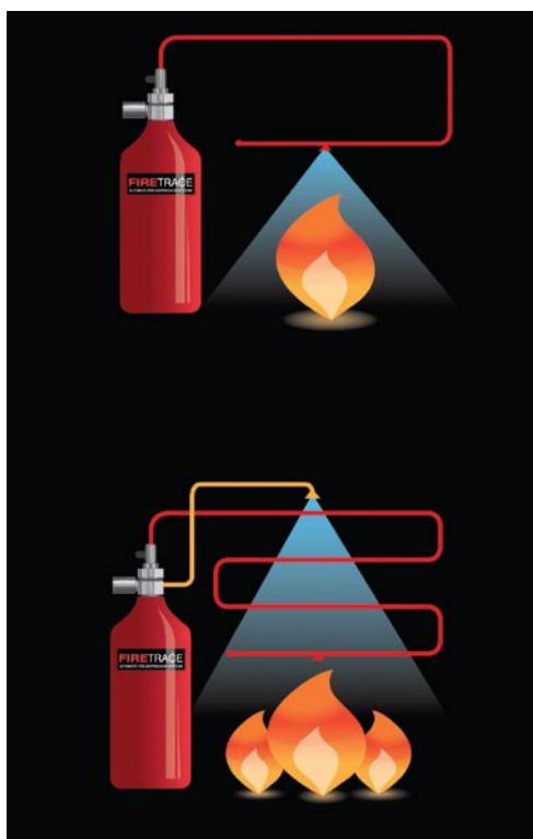
Fig. 3: A schematic diagram of the Firetrace system.
