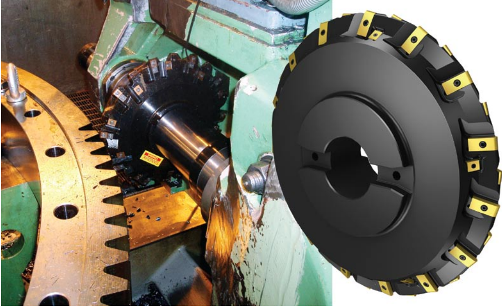
Fig. 3: In an application involving the production of 200 slewing rings per year, new PVD-coated grade GC1030 increased the productivity rate by 30% through higher cutting data capability and higher machining security through advantageous wear development.
