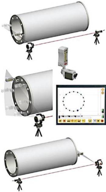
Fig. 6: The system can be used to measure the parallelism of two flanges.
