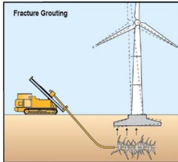
pressure of the fracture grout breaks through the annulus, permitting it access to the soil. Once the hydro-fracture pressure of the soil is exceeded, fractures open up in the soil and are immediately widened by the subsequent grout.
