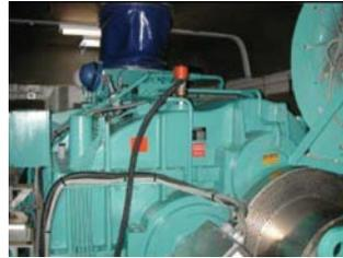
Fig. 2: An oil inlet on top of the gearbox for the return hose from the filtration unit.
