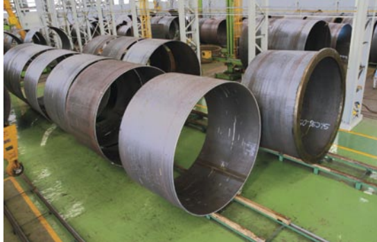
Fig. 1: Tower sections in production on the shop floor.
