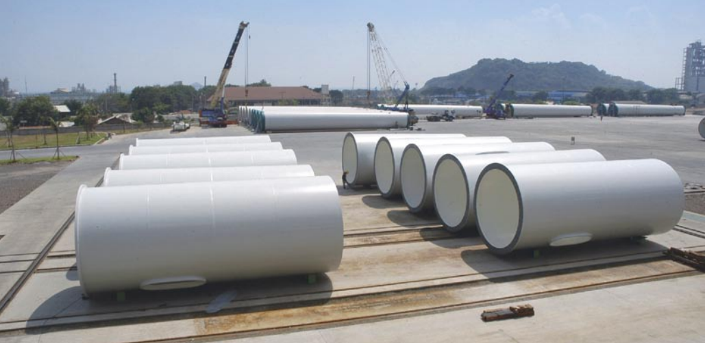
Fig. 3: Tower sections awaiting packaging.
