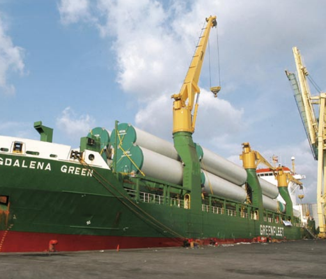
Fig. 5: Secured tower sections prepared for shipping.
