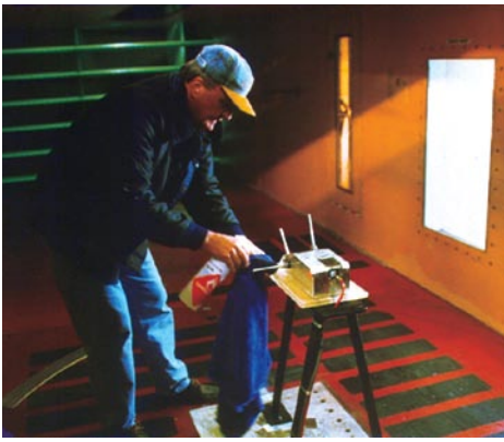
Fig. 6: Model 9734 ice sensor systems for wind power are optically the same as Model 9732 aerospace probes tested in the world's largest icing wind tunnel (at top) and used for unmanned aerial vehicles (bottom).
