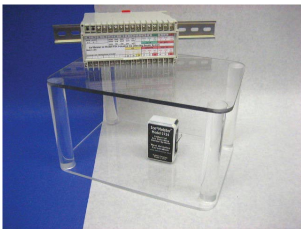
Fig. 5: Protective polycarbonate plastic cage helps shield sensor probe from damage due to melting ice falling from a stationary blade as it heats up and sheds ice.
