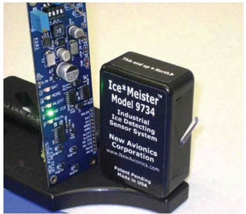
Fig. 1: Optical ice sensor for wind power turbines has no moving parts. It works on the interaction between photons of light and molecules of H 2 O.
