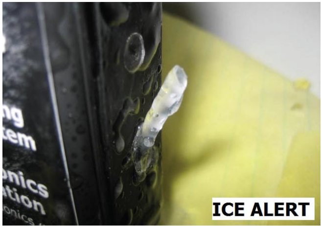
Fig. 4: Ice sensing element uses low cost infrared lasers, receivers, and fiber optics borrowed from the telephone industry to simplify manufacturing, reduce parts count, eliminate moving parts, slash cost, and make a more practical ice detector.
