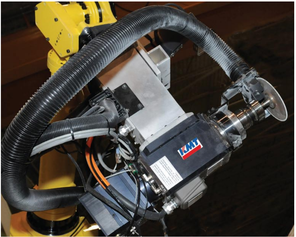
Fig. 3: A robotic router with a saw blade for edge trim.
