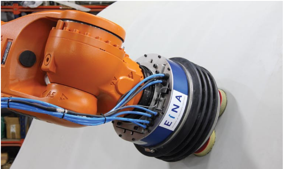
Fig. 2: A patent-pending robotic surface grinding device.
