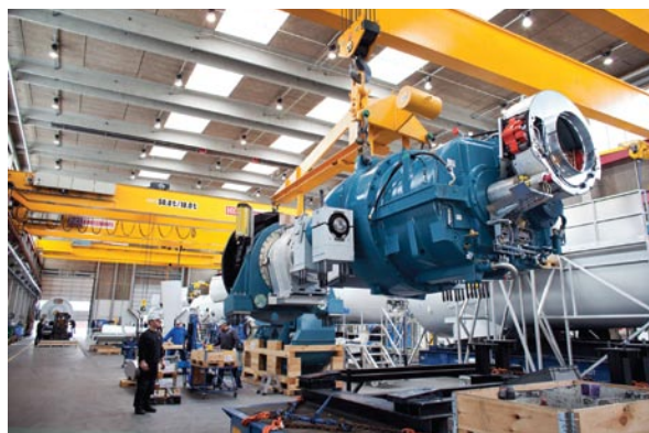
Fig. 2: The whole interior of the nacelle, including the main bearing, main shaft, gearbox, brake disc, coupling, generator, power unit and service crane, is lifted up into the nacelle behind.
