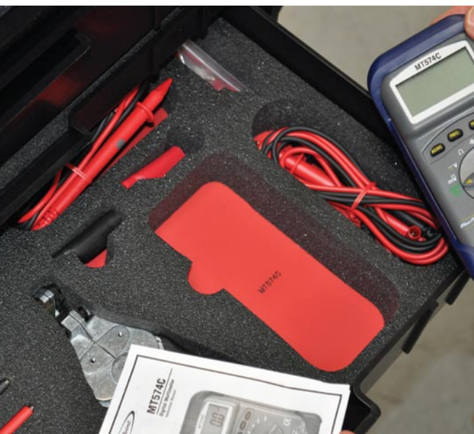
Fig. 3: A custom kit can be developed to house all the necessary tools required to perform preventive maintenance on specific components.
