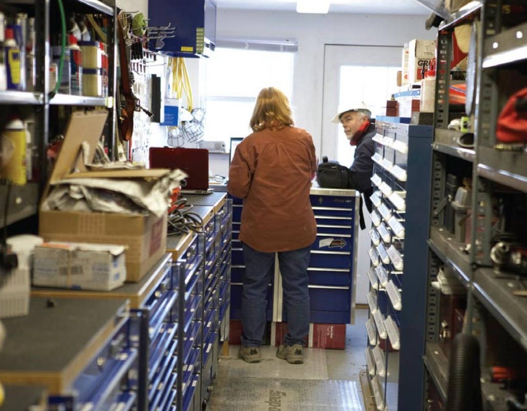
Fig. 2: Modular in design, mobile tool cribs include storage and control systems, cabinets and shelving, plus electrical components that include lighting, air conditioning and electronic keyless entry systems.
