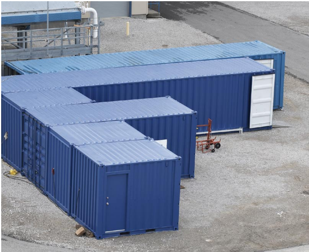
Fig. 4: Mobile tool cribs house all tools and equipment, typically in conex-type containers of 20 to 40 feet in length. All tools housed inside have been specified by the customer.
