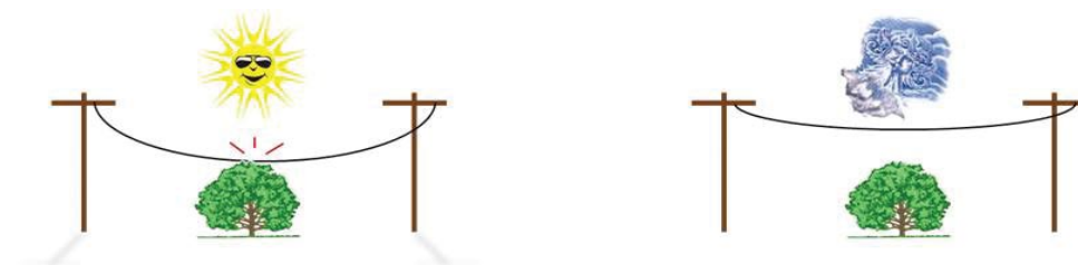
Fig. 4: Sag in transmission lines.
