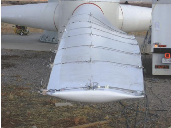
Fig. 5: An array of sensors is positioned on the turbine blade for simulation model validation study.
