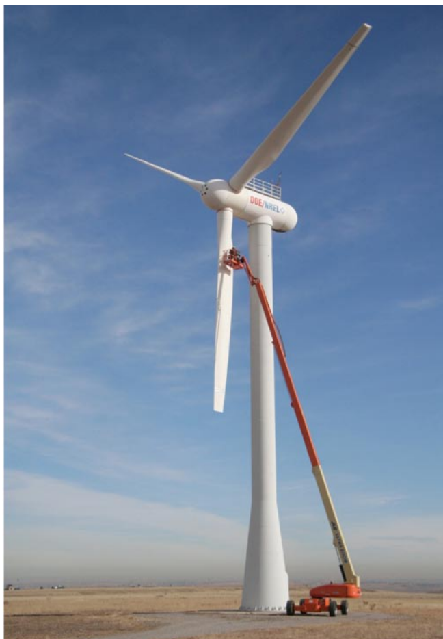
Fig. 4: For a modal survey, an engineer positions accelerometers on the blade of a 600-kW wind turbine with a 40-meter rotor diameter.
