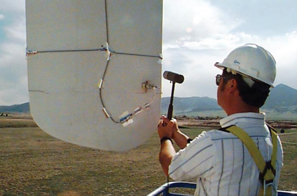
Fig. 6: An engineer hits a turbine blade with an instrumented hammer to excite the structure to vibrate.
