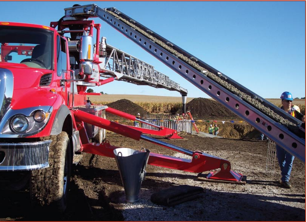
Fig. 2: Outriggers stabilize the truck during operation.
