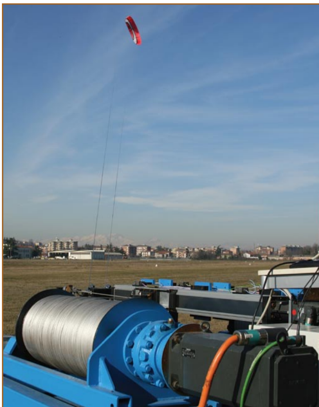
Fig. 5: The 40 kW experimental prototype, right, has been tested with tether lengths up to 3,000 ft (image: KITEnergy).
