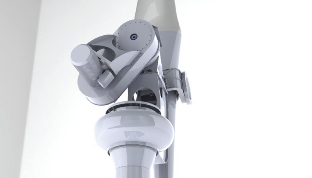
Fig. 4: The ADES pendular wind turbine employs a downwind construction shape that automatically orients itself toward the wind by means of three passive mechanical systems: a swiveling single-blade rotor, a pendulum power train, and a self-steering nacelle.
