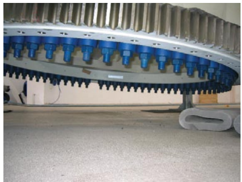
Fig. 1: A critical bolted joint found on windmills.
