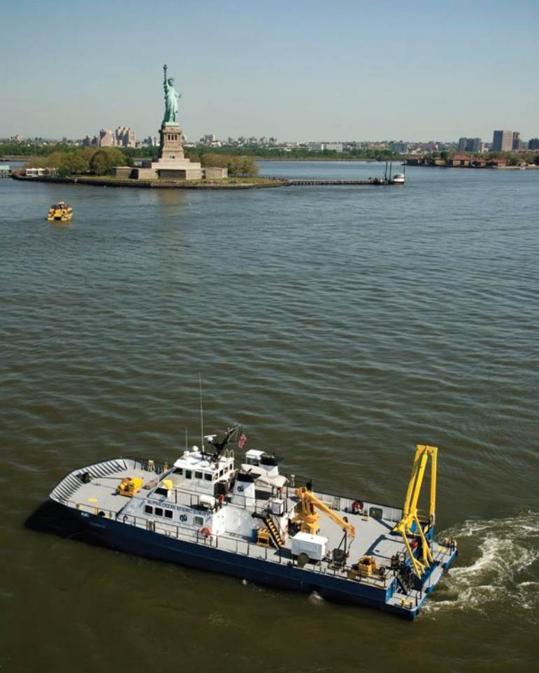
Fig. 3: The Shearwater was designed to work in marine conditions ranging from turbid coastal waters, rivers, and bays to deeper waters offshore.
