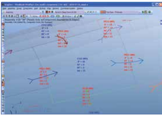
Figure 4: This screen shot illustrates the detailed composite characteristics that are optimized in HyperSizer. The blue numbers indicate the number of plies of varying fiber orientation (0, 45, and 90 degrees) within the stack. The red numbers indicate the ply drops across the zone transitions
