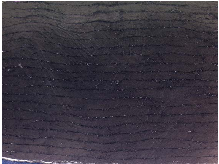
Figure 4: A laminate manufactured using Airstream™ Coating Technology at +38°C. Void content <1.5%.
