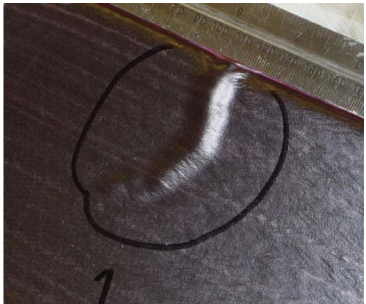
Figure 3: A Wrinkle in a carbon laminate after consolidation
