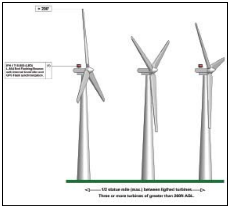
Figure 2: WindTurbine farm with IFH-1710
