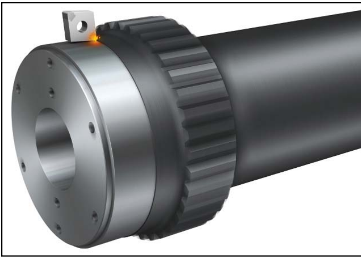
Fig 3: Hard part turning is now optimized through new combinations of CBN grades, cutting edge designs and an exact, stable insert location.
