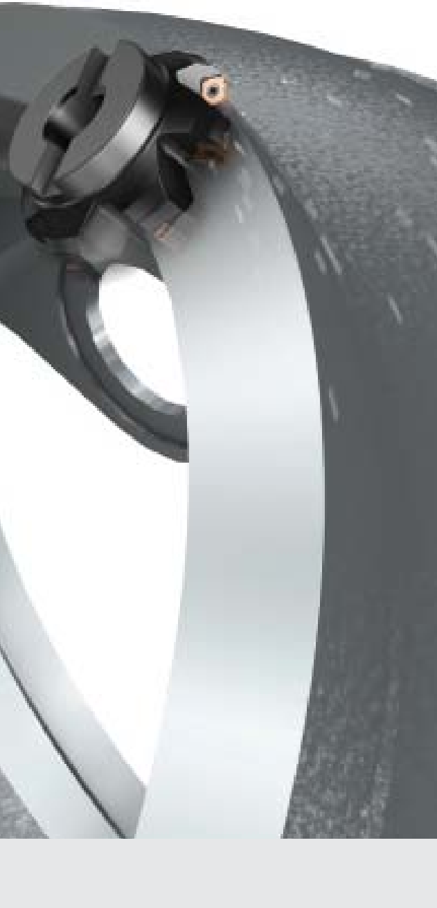
Fig 1: High feed rate with soft cutting action is ideal for milling hubs and housings.
