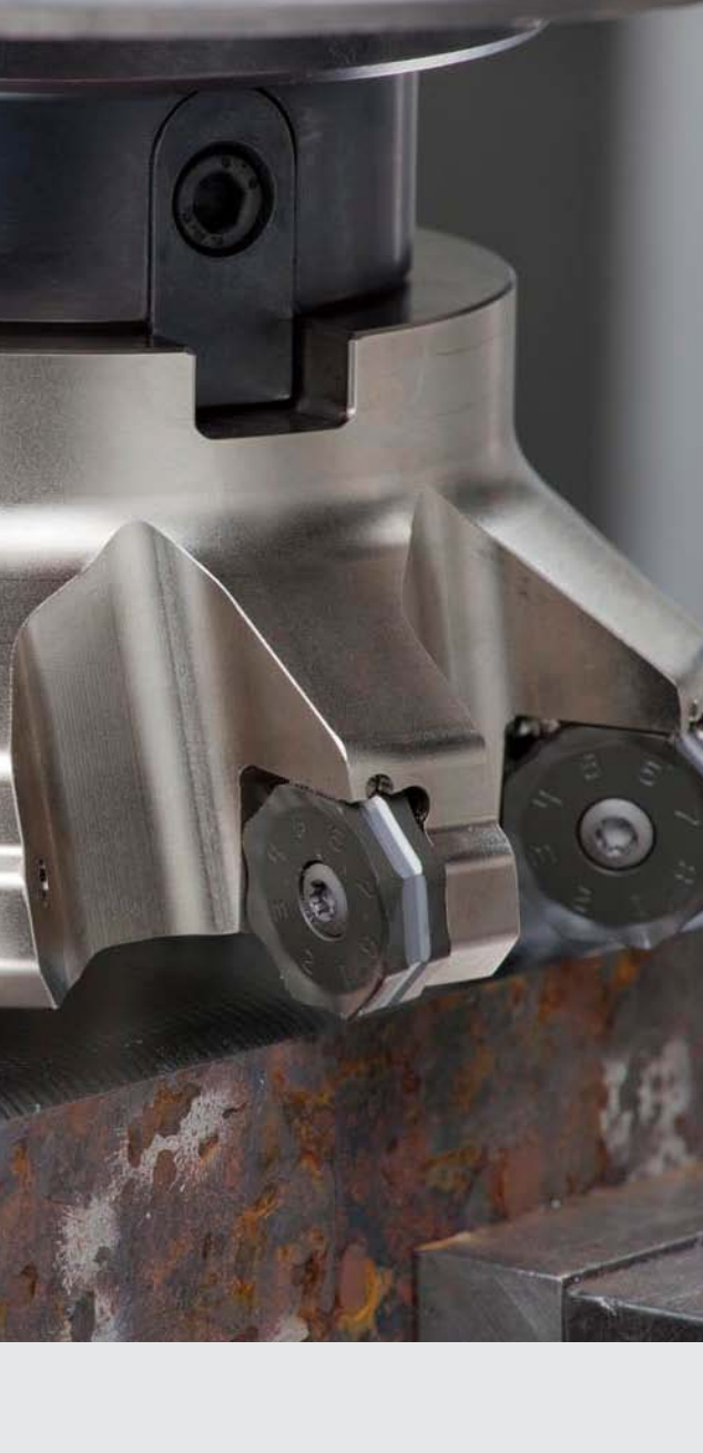
Fig. 1: Seco's Double Octomill features 16 cutting edges and provides excellent cost effectiveness.
