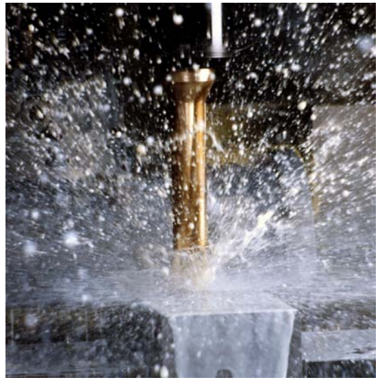
Fig. 2: A Seco Performax indexable insert drill in action.
