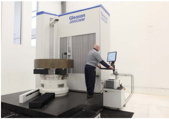
Fig. 3: New Gleason 3000GMM analytical gear inspection system speeds and simplifies the critical quality verification process for any gear, enabling Brevini to keep pace with its new gear production machines.
