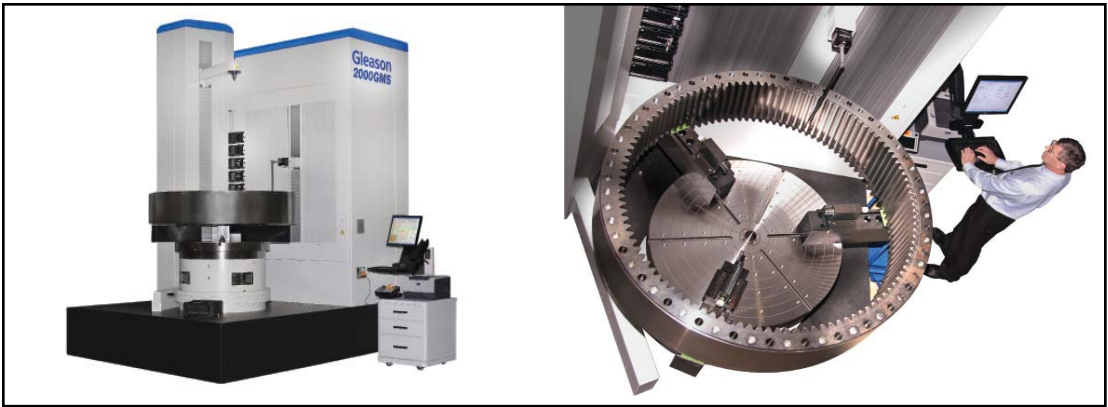
Fig. 6: Talleres Guibe's New Gleason 2000GMS performs the complete inspection of increasingly complex gear geometries up to 25% faster, while meeting VDI/VDE Class 1 specifications.
