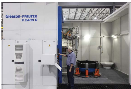
Fig. 2: New Gleason P 2400 large hobbing (top) and profile grinding machines (bottom) perform complete cutting and hard finishing operations on a new generation of very high quality internal ring gears, sun and planetary gears for Brevini's main drive gear boxes.
