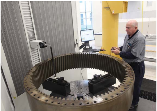
Fig. 4: “Stirring in” setup time is greatly reduced with Gleason’s Journal Reference software, which takes minutes, even hours out of the time usually required to ‘true up’ large gears manually.
