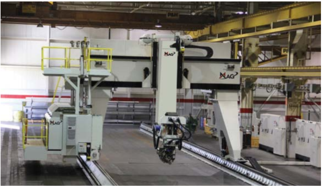
Fig. 2: Unidirectional towpreg processing in a flat tool via automated fiber placement machine (photo courtesy of MAG).
