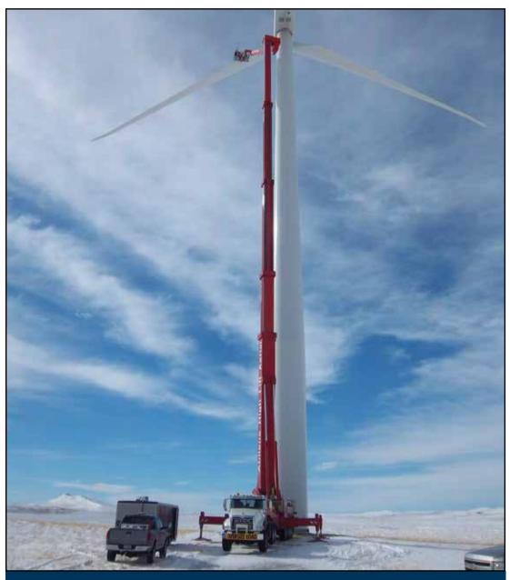
With a maximum height of 328 feet and stable enough to operate in 35 MPH wind, Abilene High Lift Aerial claims its Ruthmann Steiger TTS 1000 is the "largest, most stable aerial lift in North America."
