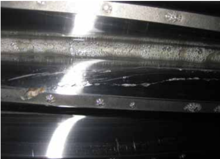
Figure 7: Visual inspection of gear show a fractured tooth.
