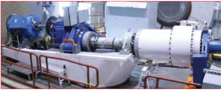
Figure 3: 750 kW wind turbine drivetrain of NREL GRC.
