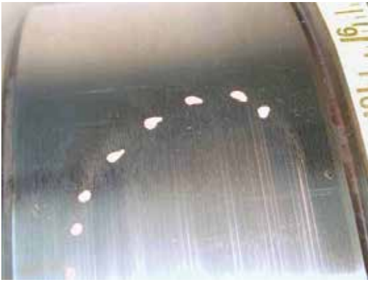
Figure 13: A cylindrical planet bearing with sliding marks in the circumferential direction [32].
