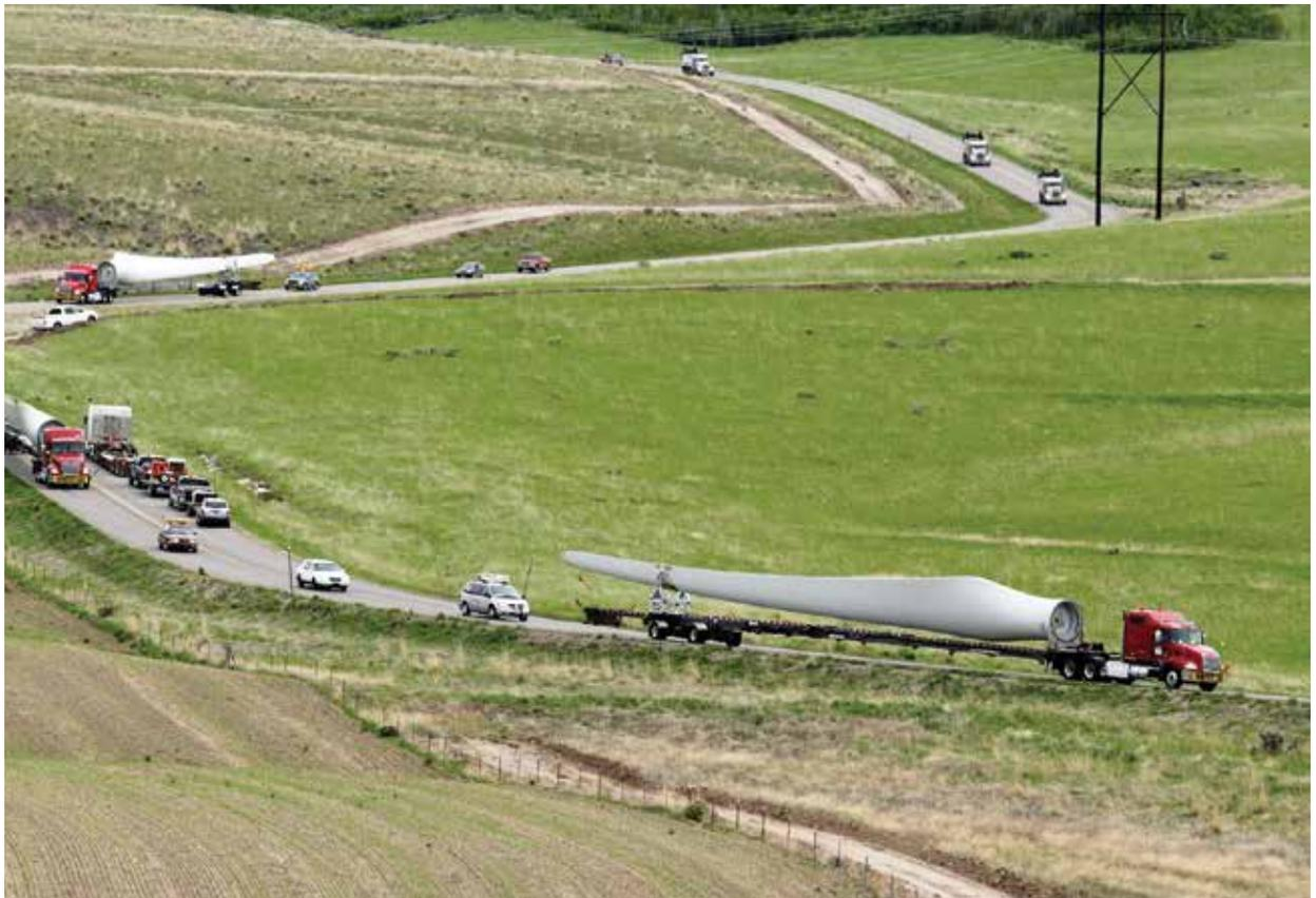
The complex logistics involved with transporting one-piece blades generally amounts to 3-5 percent of the total installed cost of each turbine.
