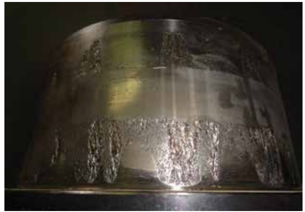
A picture of the damaged rotor side intermediate bearing inner race.
