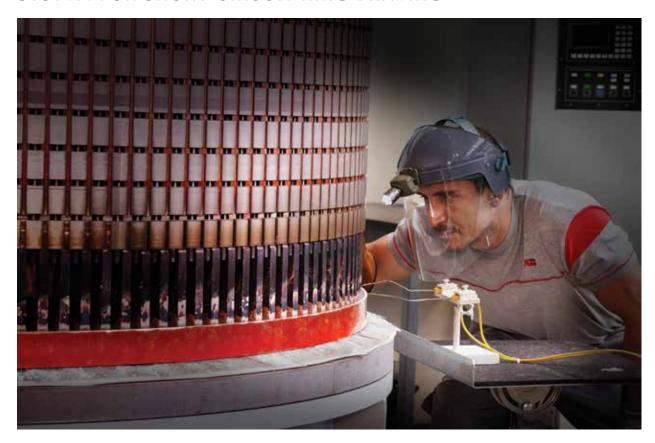
Power generation and distribution giant ABB recently installed the largest single-shot shortcircuit ring brazing system yet developed by EFD Induction. The system, which was installed at the ABB plant in Vittuone outside Milan, Italy, can braze rings with a diameter up to 1,500 mm.
